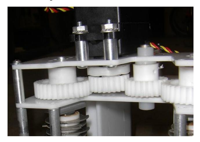
Capture gears between the standoff plates.
