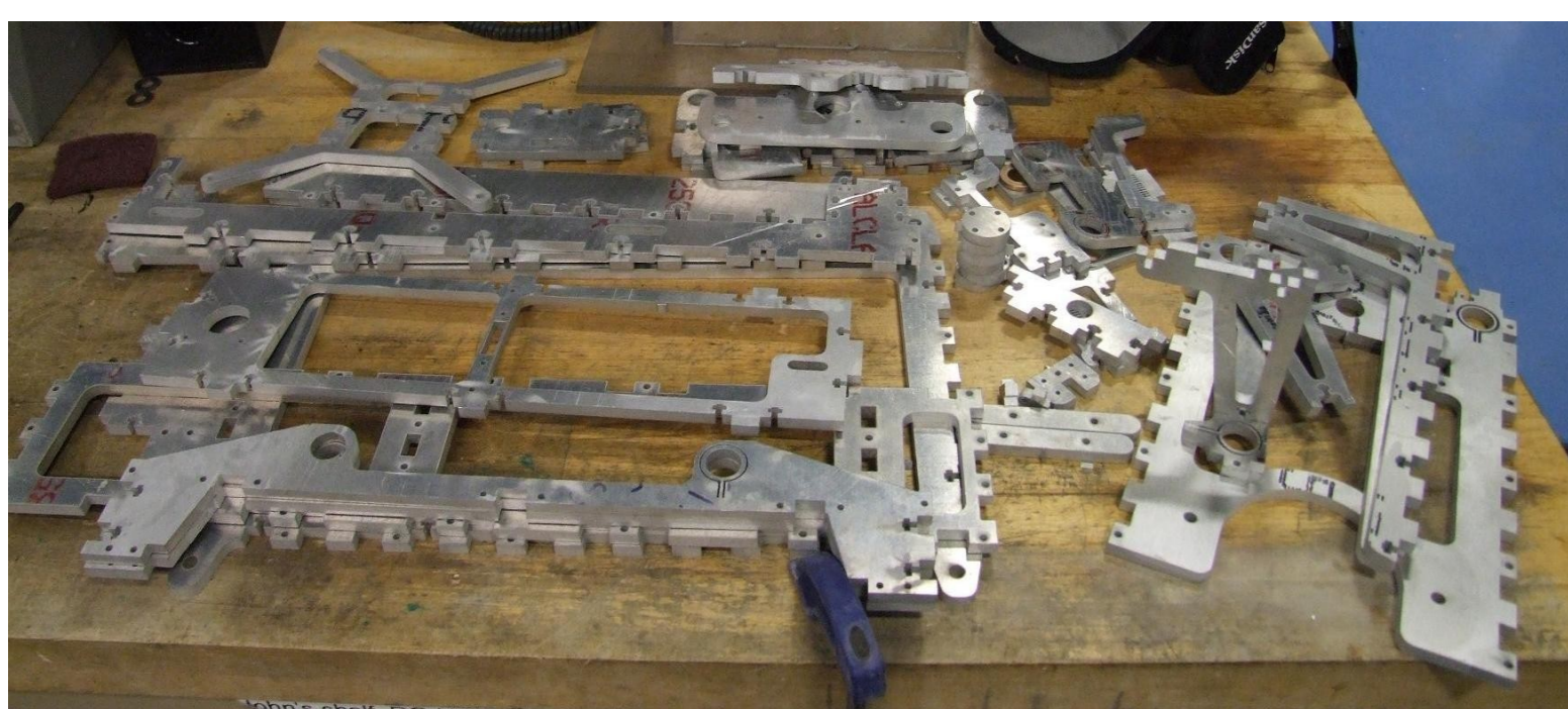
Above: The parts of FABulus were made on a campus abrasive waterjet cutter
