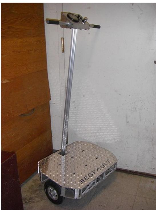
**Segfault** is a custom two-wheeled self-balancing vehicle similar to the Segway Personal Transporter. However, it is unique from other custom Segway-like vehicles because it uses no digital logic in its balancing controller. While the Segway and other amateur replicas use digital microcontrollers to read and process the sensors, in Segfault, all of the signal processing is represented by analog voltages.
