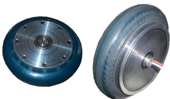
These motors are all of the *permanent magnet synchronous* topology, commonly called “Brushless DC” motors. These motors do not have the complex carbon brush mechanics found in a DC motor. Consequently, they must be controlled with an electronic *inverter*. Despite this requirement, they are capable of higher efficiency and power than a DC motor. They can therefore produce useful torque at small scales.
