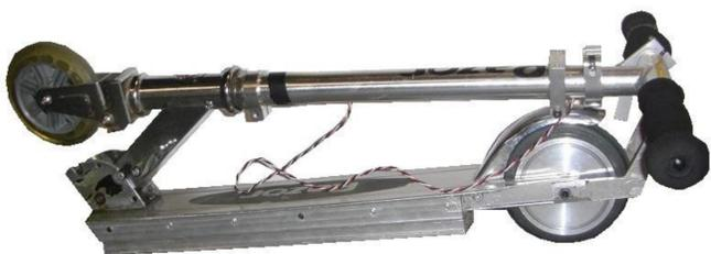
The first hub motor scooter, “RazEr”, weighs only 6 kg and can travel at 20 kph
