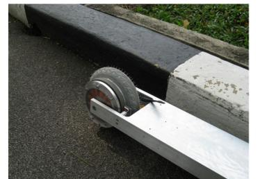
“Pneu Scooter” is an experiment in using pneumatic tires with hub motors.
