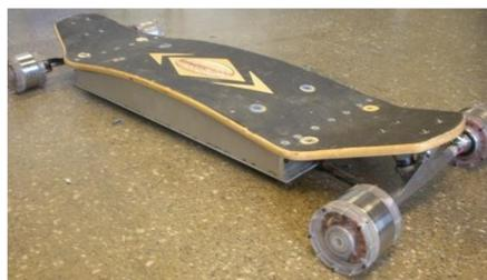
The Electric Longboard has four 500 watt brushless hub motors
