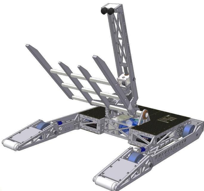
30 lb class robot **Überclocker Remix** uses a unique double-actuated lifting fork to both clamp down and lift opponents for total control.
