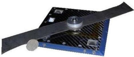
**Pop Quiz**, a 1 lb class robot with a horizontal spinning titanium impact bar
