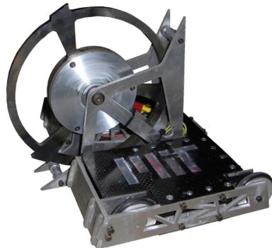
**Nuclear Kitten 5** is a 3 lb class robot with a vertical spinning toothed disc
