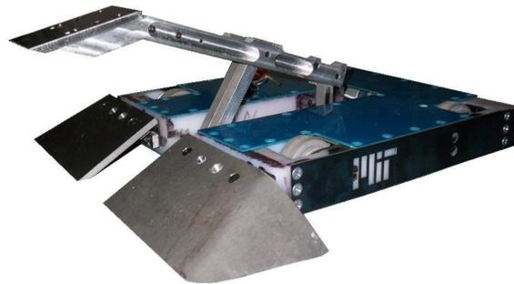
**Test Bot** is a 12 lb class robot with an electric lifting arm using a 4-bar linkage
